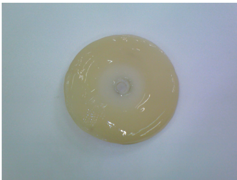
Fig. 7. Photograph of bacterial cellulose membrane formed on the surface of the disk during the fermentation using a RBC.
